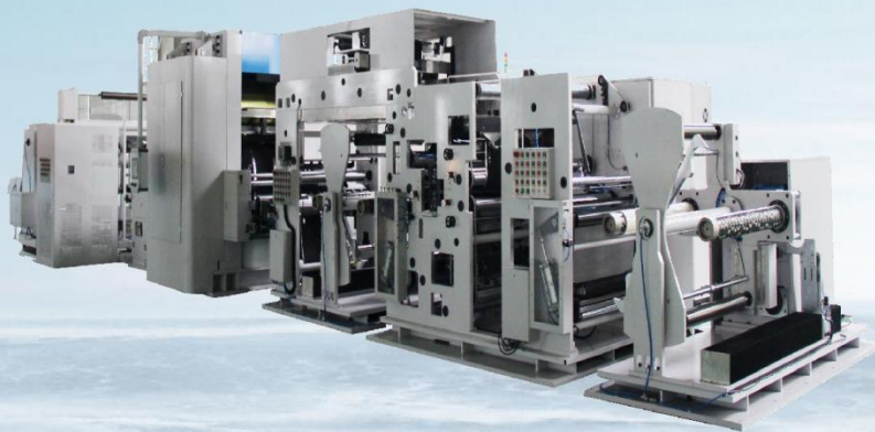
Product Model: SD750-W1100-ZQ Automatic Rolling Slitter Machine
